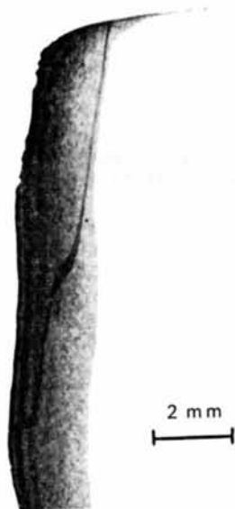
Fig. 4. Lang topograph of crystal A . The edge is parallel to the (220) reflecting planes. The germanium 220 reflexion and Mo K\alpha_1 radiation were used.
